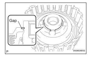
(b) Install the No. 1 clutch balancer and forward clutch return spring sub-assembly.
