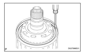
(b) Using a screwdriver, install the snap ring onto the clutch drum and input shaft assembly.
