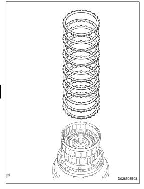
(b) Remove the reverse clutch flange, 6 plates and 5 discs from the clutch drum assembly.
