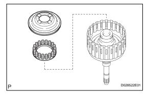
(b) Remove the No. 1 clutch balancer and forward clutch return spring from the input shaft assembly.
