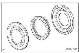
(e) Remove the No. 2 clutch balancer and direct clutch return spring sub-assembly from the direct clutch piston sub-assembly.
