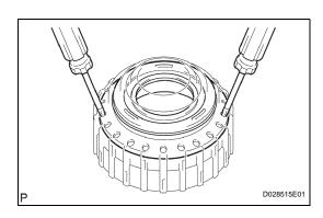
(c) Using 2 screwdrivers, remove the direct clutch piston sub-assembly from the clutch drum.
