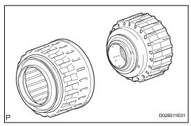
(c) Be careful not to damage the O-ring. Press in the clutch drum sub-assembly into the reverse clutch piston with both hands.
