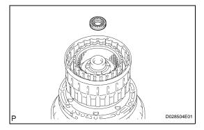
(b) Install the thrust needle roller bearing onto the clutch drum assembly.
